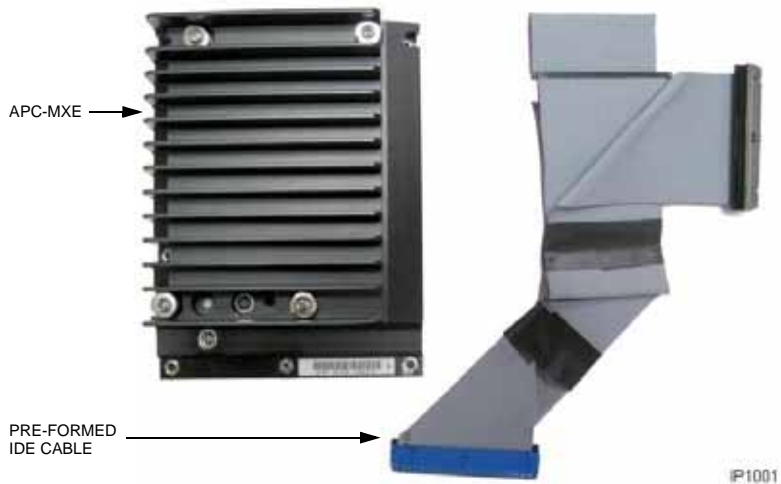
Figure 31: APC-MxIII and Pre-formed IDE Cable
