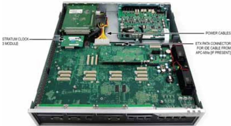
Figure 33: Removing the Power Cable
