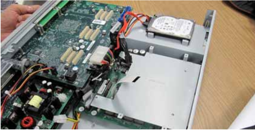
Figure 49: AOB Mounting Plate in Position
