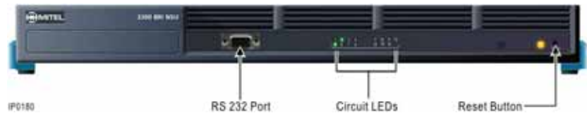
Figure 112: BRI NSU – Front Panel
