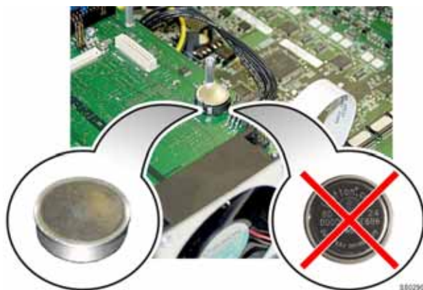
Figure 40: Installing the System i-Button
