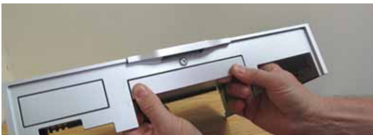
Figure 46: Remove Blanking Panel
