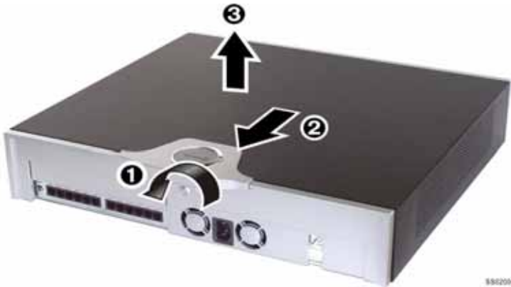
Figure 11: CX/CXi, CX II/CXi II - Removing the cover
