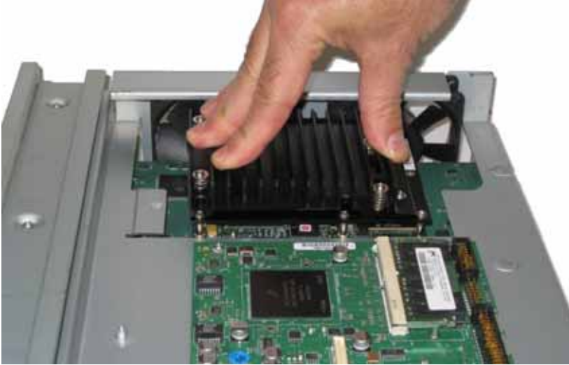
Figure 53: Installing an APC-MXe in the MXe Server
