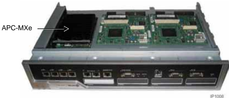
Figure 51: APC-MXe on MXe Carrier Board
