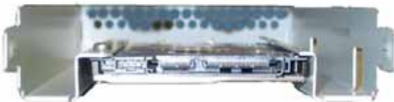
Figure 75: Hard Drive / SSD Installed in Drive Carrier
