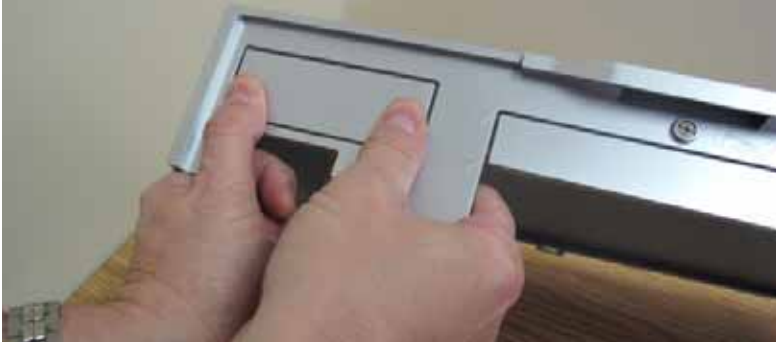
Figure 66: Remove Blanking Plate
