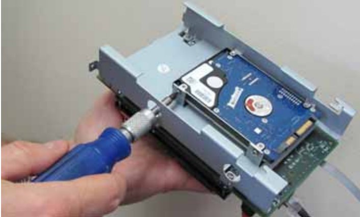
Figure 67: APC-CX(i) II Hard Disk Drive Removal
