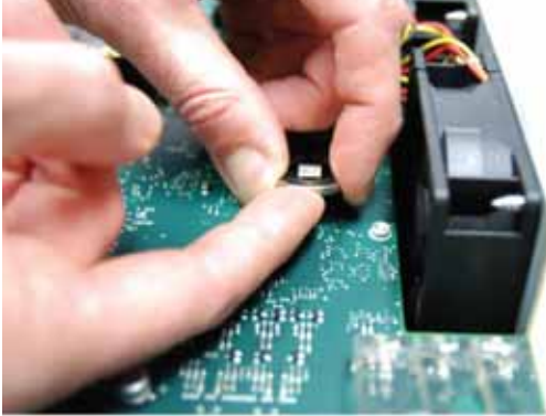
Figure 54: Removing the Battery
