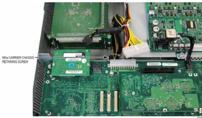
Figure 34: Carrier Chassis Retaining Screw
