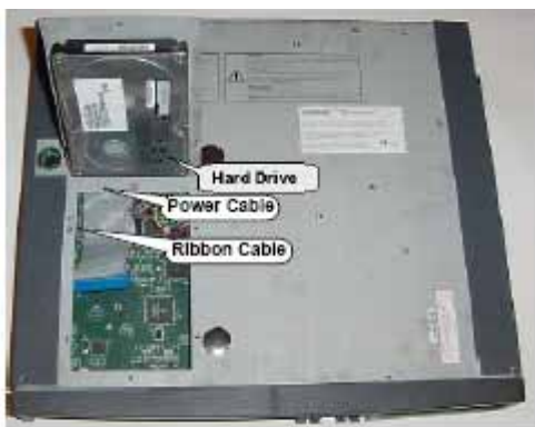
Figure 74: LX Controller Hard Drive Installation
